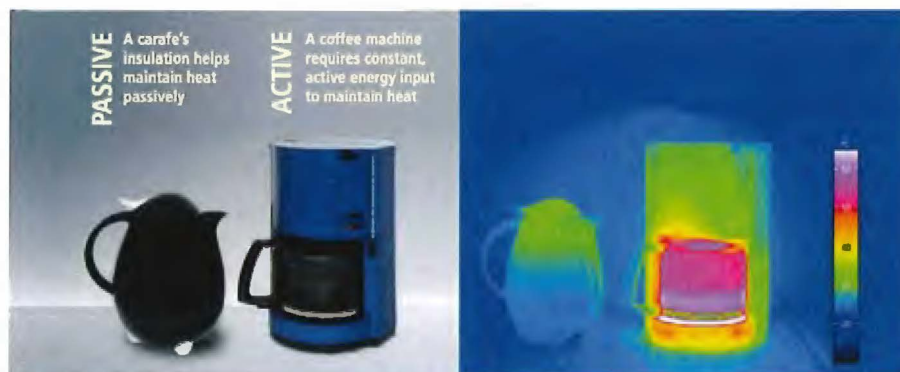
Figure 1 – Passive vs Active: Good thermal insulation reduces the need for active heating; likewise, a properly insulated building envelope can minimize the need for active heating. The thermograph on the right shows hot spots in the “active” system, where heat loss occurs at the greatest rate. [Source: Passive House Institute]
