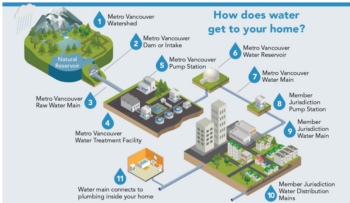
Metro Vancouver Watershed and Water Transmission Map
