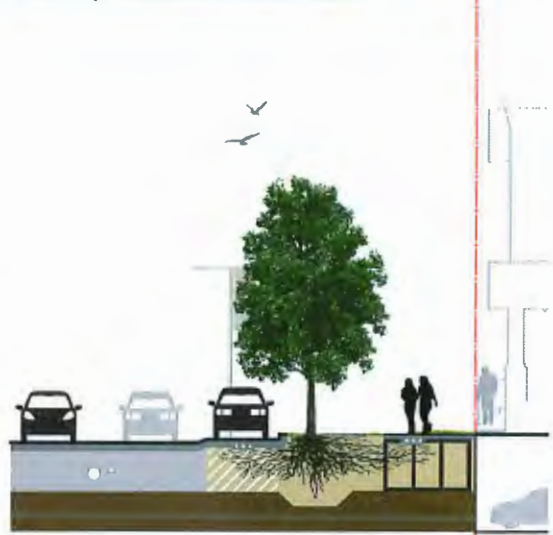
“ENGINEERED” | OPEN VOLUME + STRUCTURAL / CONSTRUCTED SOIL VOLUME
