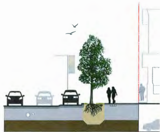
“TYPICAL” | INADEQUATE SOIL VOLUME
