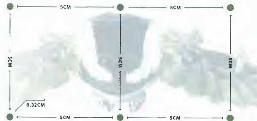
FIG 1 Diagram of bird friendly glazing pattern with visual marker, at maximum 5cm x 5cm spacing IMAGE SOURCE: FLAP CANADA
