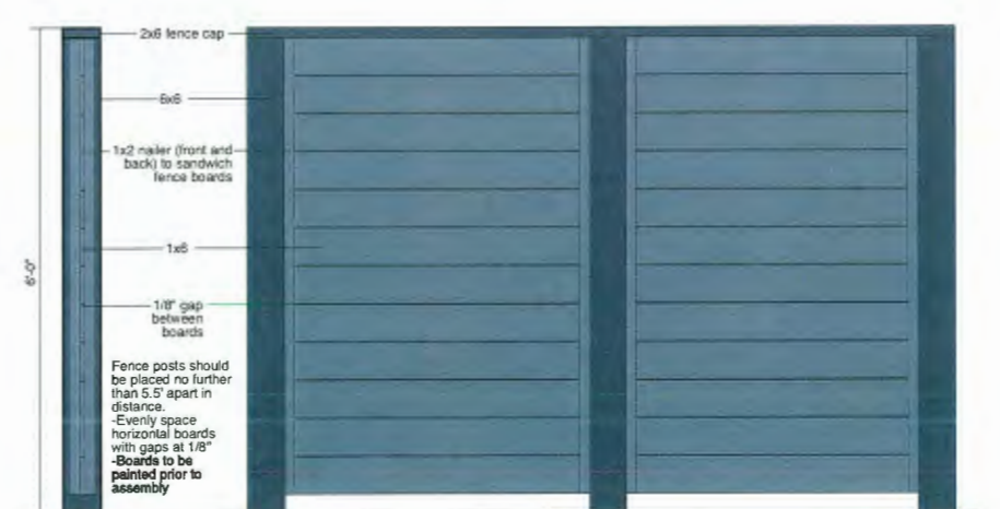
L4-14 ROOF LEVEL - Wood Privacy Fence (6'-0" H) Cedar - Screening around Mechanical Equipment Scale: 1"=1'-0"
