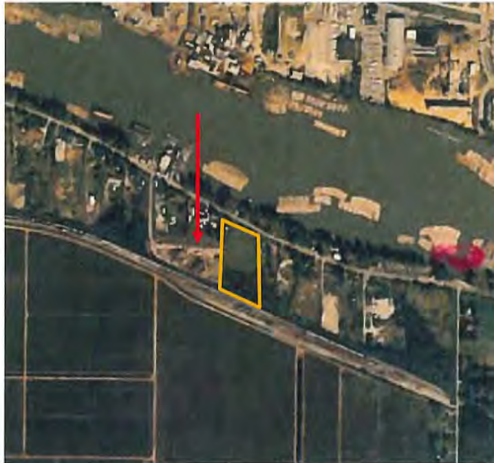
PHOTO 9: AIRPHOTO FROM 1997 SHOWING ACTIVE SOIL FILLING TO THE WEST (RED ARROW). THIS MATERIAL WAS PLACED SEVERAL METRES HIGH AND IS NOW OVERGROWN WITH BLACKBERRY. MR. SAHOTA'S PROPERTIES (BOTH THE SITE AND 17260 RIVER ROAD) ARE OUTLINED IN ORANGE.
