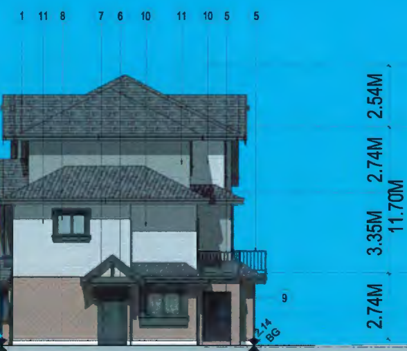
4 BUILDING C NORTH ELEVATION SCALE 1/8"=1'-0"
