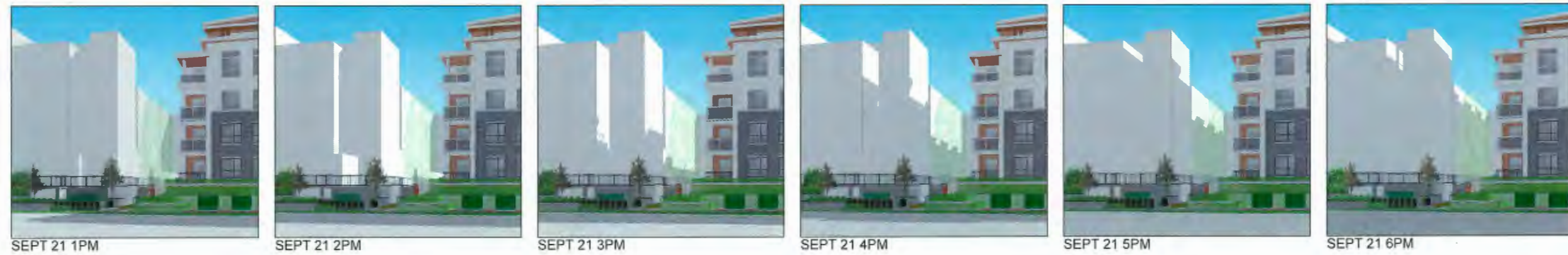
SHADOWING ON REMY WEST FACE (NORTH END, CAMBIE ROAD) - AUTUMN EQUINOX (1PM TO 6PM)
