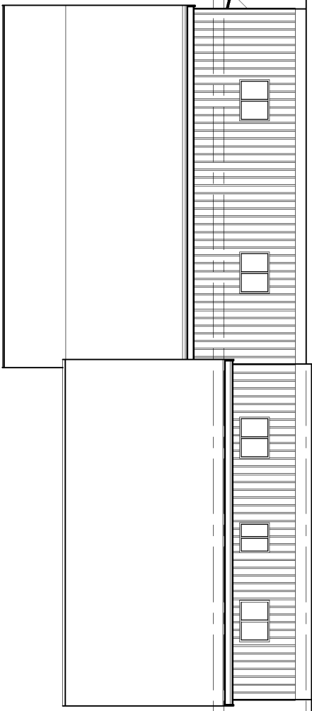
South Soffit above windows for 1.2m on each side shall be protected with non-combustible material
