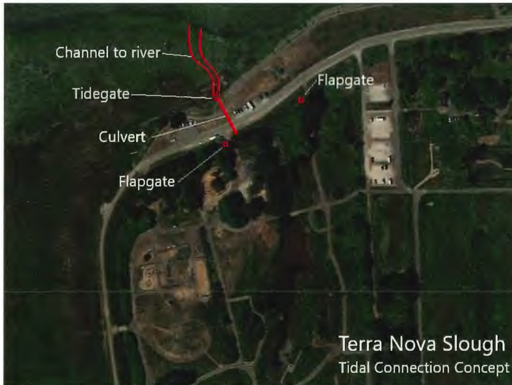
Figure 4: Option 1 – Floodbox with Self-Regulating Tide Gate
