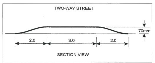
Typical Dimensions of Speed Hump (as proposed)
