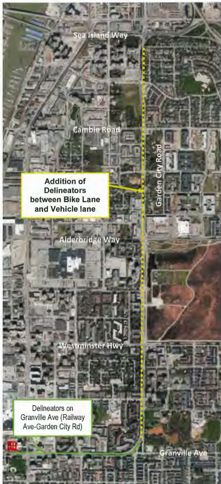
Garden City Road (Granville Ave-Sea Island Way): Addition of Delineators between Bike Lane and Vehicle Lane
