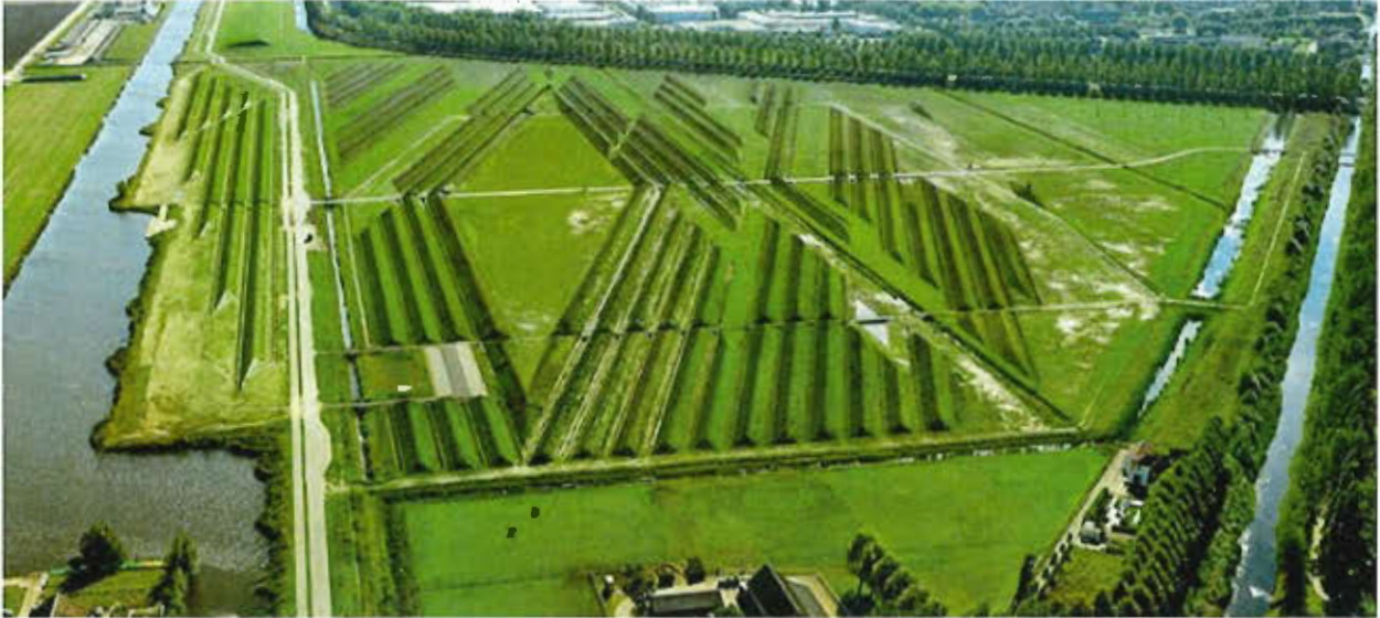
Figure 2: 80-acre green space adjacent to Amsterdam Schiphol Airport with landscaping to deflect noise
