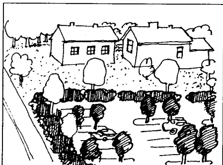
Screen parking with min. 2.0m wide by 1.5m high landscape strip. One tree should be planted for every four cars.
