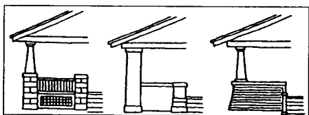
Some typical porch supports and porch railings
