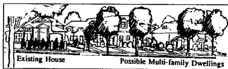
A smooth internal conversion can be achieved by using typical single-family forms and massing in the design of new multi-family dwelling
